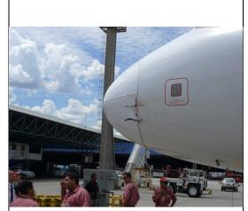
In the picture there is a plane standing on the apron in front of the terminal. The radome of the aircraft is damaged and we can assume that it is due to a bird strike. There are ground crew specialists by the airplane. They are inspecting the radome and estimating how big the damage is.
